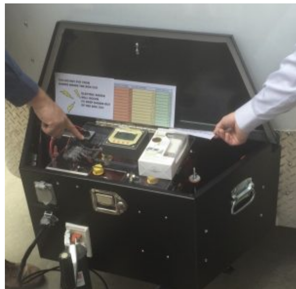
Figure 1. Tongue-mounted power distribution box
